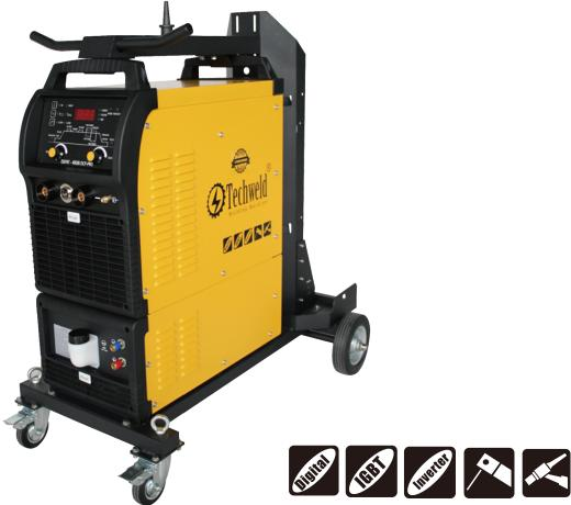
EXPAT - 4000i DCP-PRO is digital DC pulse TIG models with MCU technology, suitable for both automation application and manual welding. DC pulse function minimize the heat input for thin materials and provide a faster freezing for uphill welding.
